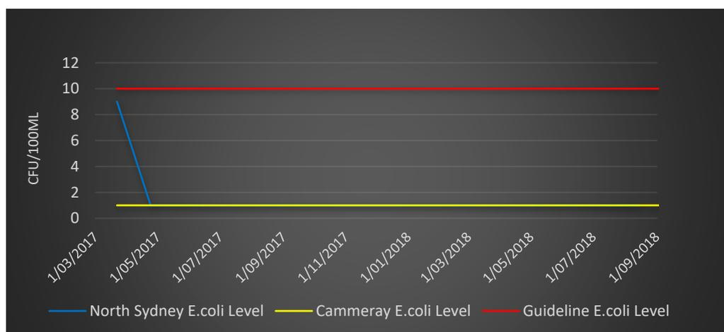
**Figure 3** E.coli Levels in Recycled Water Produced at the Two Major Treatment Points in the Scheme
