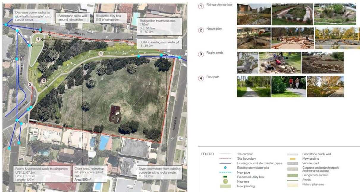
**Figure 3: An example concept design option showing the integration of the treatment system into an holistic park upgrade.**
